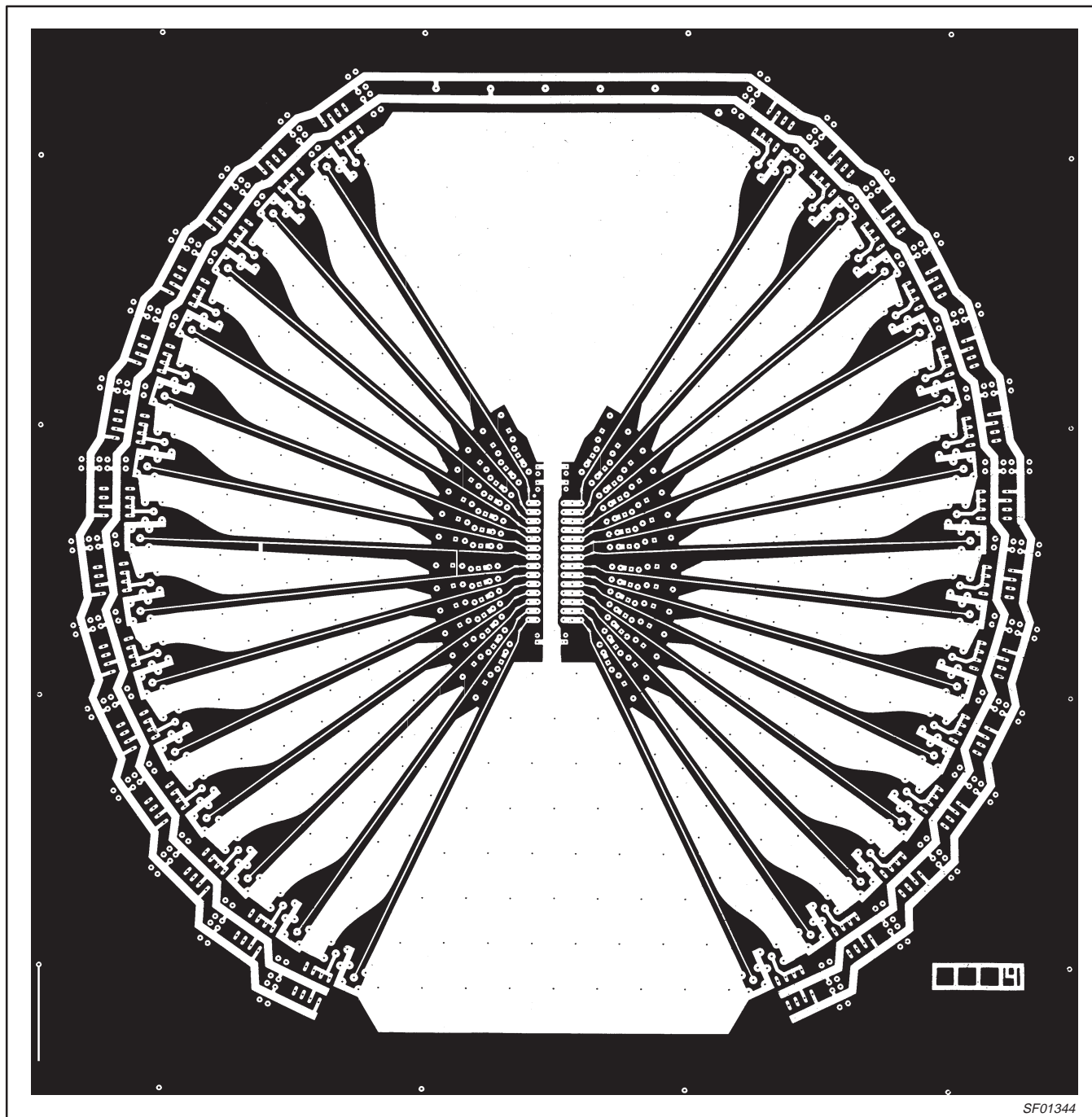
Figure 3. Board Layout — Bottom Side
